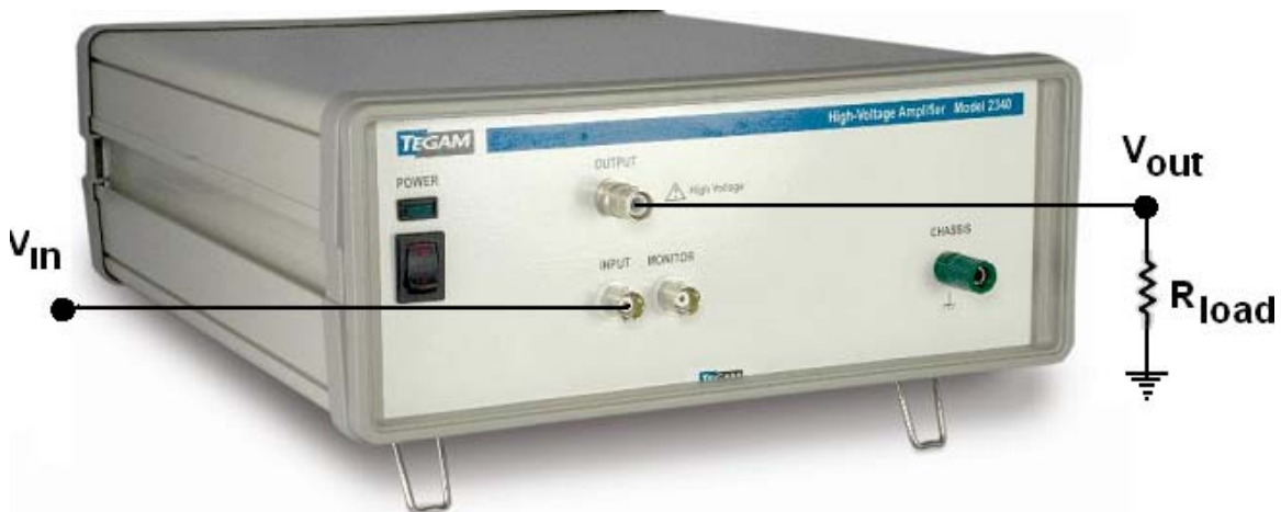
Figure 3 - A resistive load at the output of the voltage amplifier.
