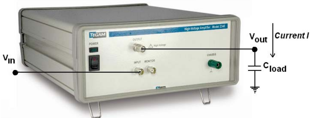
Figure 4 - A capacitive load at the output of the voltage amplifier can change its slew rate.
